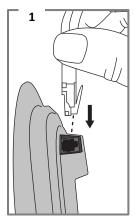
Ensure the clip is firmly connected. A click should be heard when inserted correctly.
