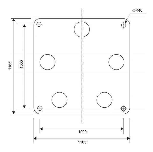
Figure 1: CardioWall Compact mounting points (Dimensions in mm)
