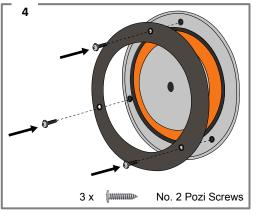
The securing ring **MUST** be fitted to the new pods.
